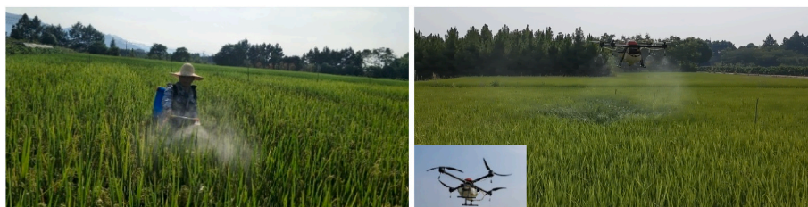
Fig. 11. The spraying operation of a knapsack sprayer and an agricultural spraying UAV in a rice paddy.
